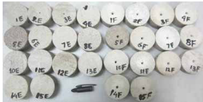
Picture 1 Discs without and with holes at the centre prepared from sandstone cores for Brazilian and ring tests respectively
